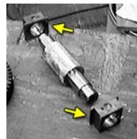
**9** Place the two compression springs into the depressions on the lower roller blocks. Then, slide the upper roller assembly into the mill, keeping the spring aligned.
