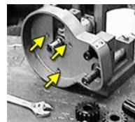
**12** Using an Allen wrench, loosen the two recessed set screws located at the back of the mill. You should now be able to slide the bronze roller blocks, along with the roller itself, up and out of the mill.
