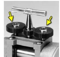
**4** With both indexing gears raised, unscrew all four hex head bolts (see photo on right) and lift the top plate off of the mill.
