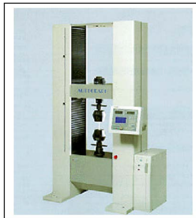
Figure 6.1. A photograph of a tensile machine (Shimadzu, Autograph AG-10TC). 2
