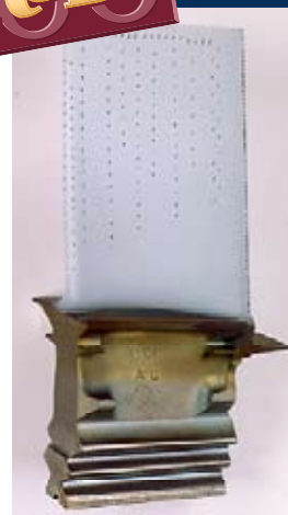
Commercial thermal barrier coating (TBC) deposit onto a Ni-based superalloy gas turbine blade
