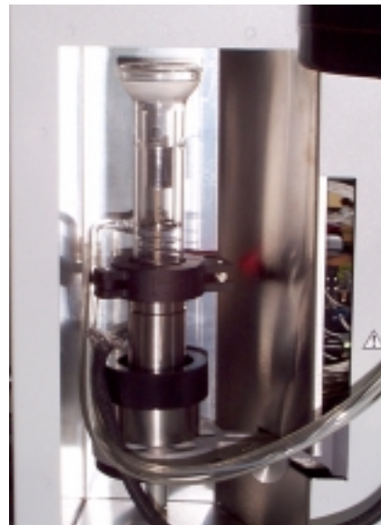
Furnace in cooling position
