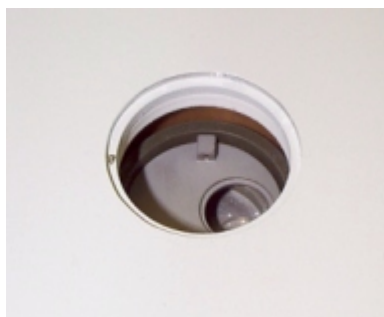
Lower furnace lid holder with lower lid removed.
