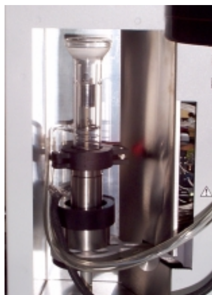
Furnace in the cooling position
