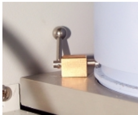
Back locking mechanism in locked position.
