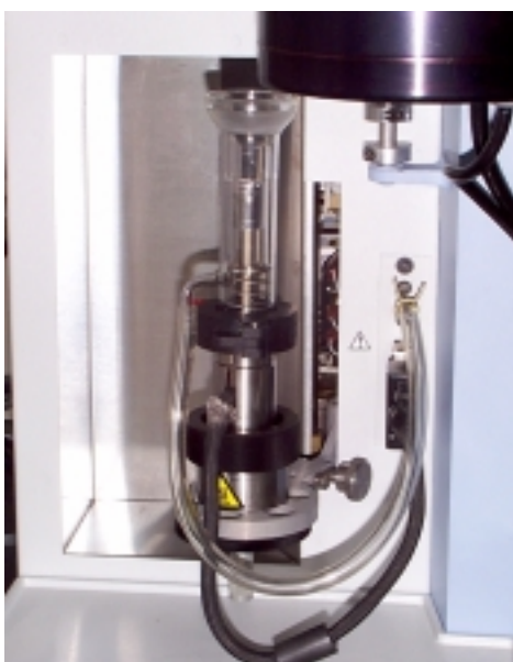
Furnace in the lowered position
