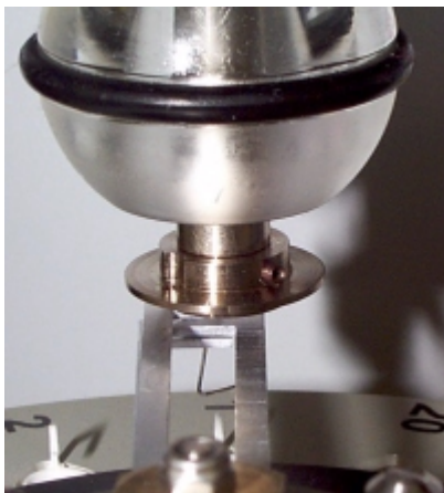
Position of the crucible after clicking on Move Left by a Small Step from the correct position. The handle moves clockwise.
