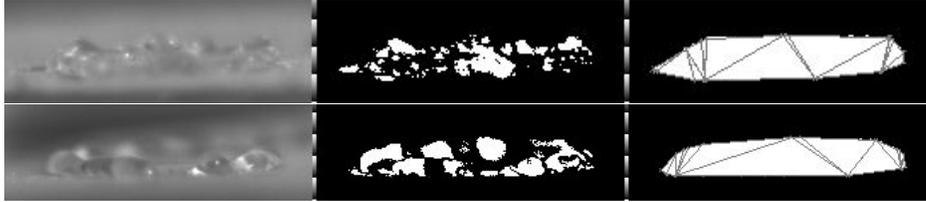
**Figure 1:** On the left, two droplets of water interacting with two different hydrophobic surfaces. The middle shows the detected droplets as per foreground detection. On the right are triangulated convex hulls.
